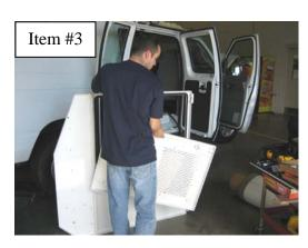
Remove **Emergency Exit Hatch** from **Front Bulkhead** to ease installation
